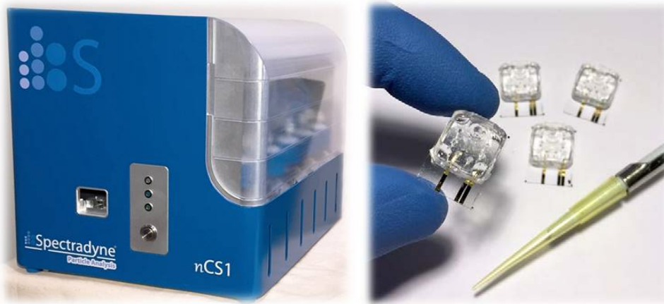
Figure 1. The nCS1 instrument and cartridges.
