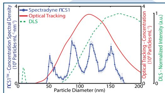
**Figure 1.** Direct comparison of Spectradyne's nCS1 with single-particle optical tracking and dynamic light scattering. Only the nCS1 reveals the true composition of the polydisperse sample, a mixture of 52, 94, 122 and 150 nm polystyrene particles.
