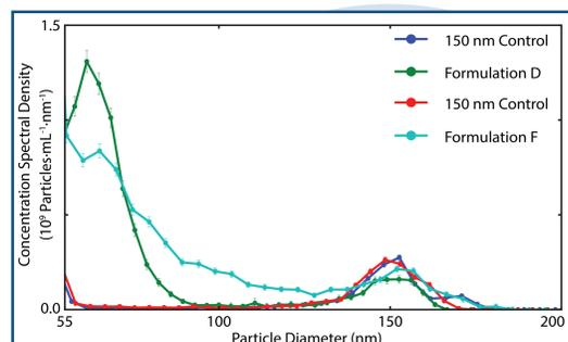
**Figure 3.** Time-dependent degradation of a cancer-targeting biocomposite nanoparticle formulation using Spectradyne's nCS1. Before (green): mean diameter 62 nm, dispersion 21%. After (light blue): broad distribution of particle sizes with no clear peak.
