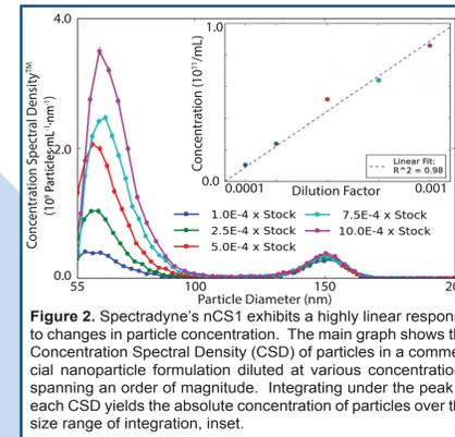
**Figure 2.** Spectradyne's nCS1 exhibits a highly linear response to changes in particle concentration. The main graph shows the Concentration Spectral Density (CSD) of particles in a commercial nanoparticle formulation diluted at various concentrations spanning an order of magnitude. Integrating under the peak in each CSD yields the absolute concentration of particles over the size range of integration, inset.
