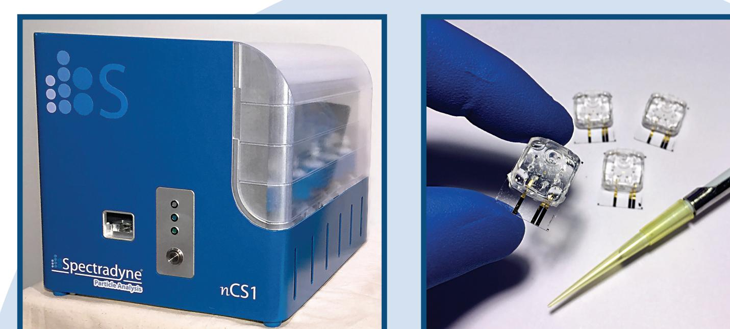
The Spectradyne nCS1 MRPS system occupies a small bench top footprint, approximately 1.5 sq ft (left). Only 3  $\mu\text{L}$  of sample is required for analysis using a disposable microfluidic cartridge (right), which prevents contamination between measurements and eliminates cleaning requirements.
