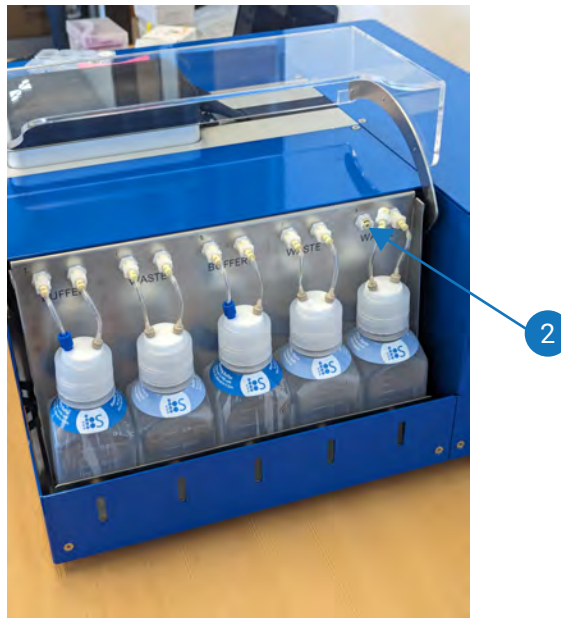
Figure 4: Disconnecting the fifth bottle's fluid line
