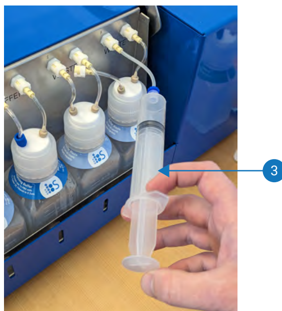
Figure 5: Connecting the bleach filled syringe to the fifth bottle's fluid line
