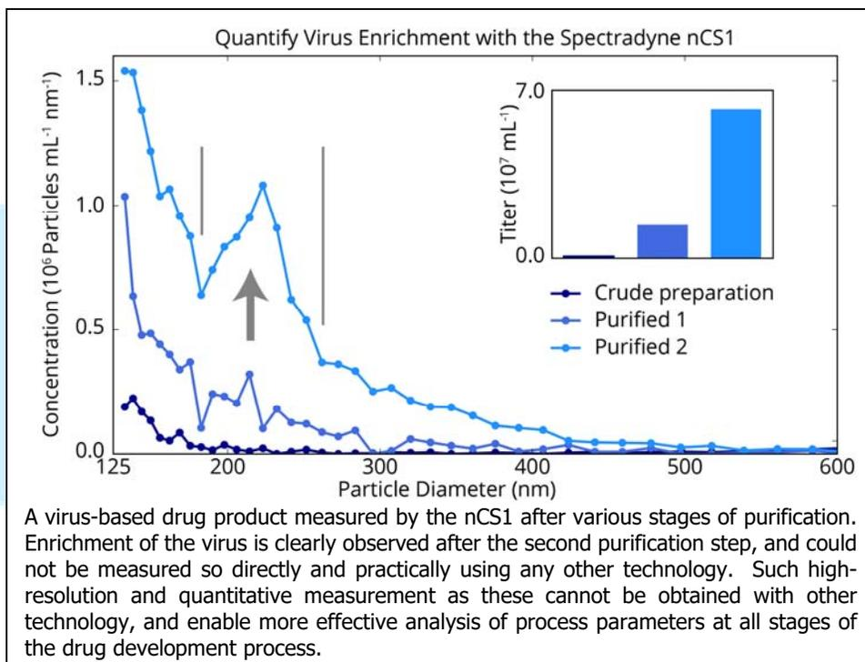
Because the nCS1 uses an electrical method, not light scattering, to count and size nanoparticles it measures all particle types equally well. As a result, researchers count on the nCS1 every day to measure diverse range of gene therapy vectors and other nanomedicines, including:
