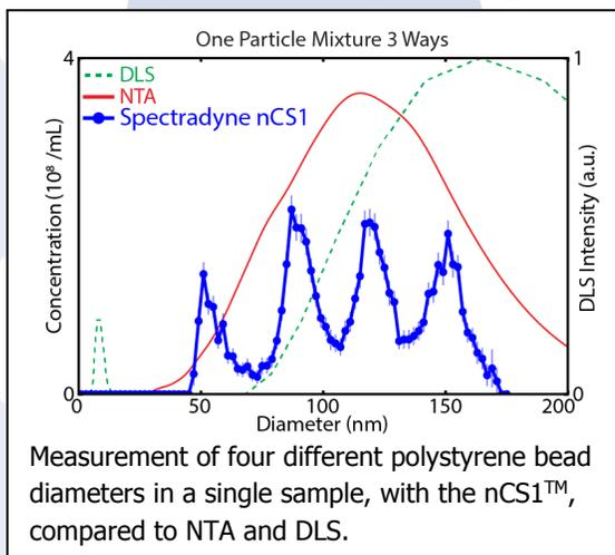
The RPS method offers much higher resolution than do methods that rely on optical techniques, such as dynamic light scattering (DLS) and nanoparticle tracking analysis (NTA). In the figure to the left, we compare measurements of a mixture of different diameter polystyrene beads measured with the nCS1™ with measurements of the same sample with NTA and DLS. The two optical techniques fail to resolve the four different particle diameters, and further give the incorrect concentration of particles.
