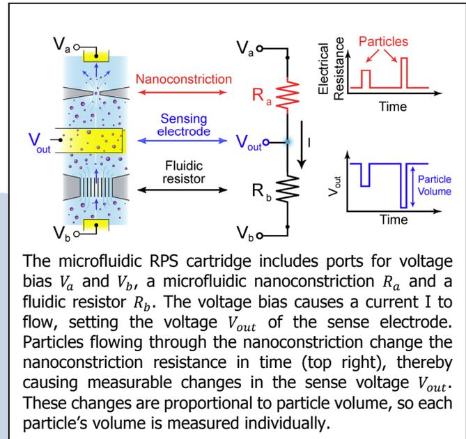
flows through the nanoconstriction, it changes the electrical resistance of the constriction by occluding part of the current, by an amount proportional to the ratio of the nanoparticle volume to that of the nanoconstriction. Individual particles thus give changes in the sense voltage proportional to their volume, allowing them to be counted and sized. The much smaller nanoconstrictions available in Spectradyne LLC's microfluidic cartridges allow much smaller particles to be detected.
