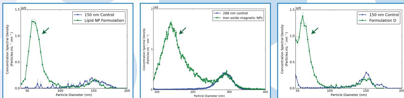
Detection of 4 different nanoparticle materials: Lipid nanoparticles (62 nm, left), iron oxide magnetic nanoparticles (140 nm, center), and biocomposite (61 nm, right) in addition to polystyrene control particles (left and right 150 nm, center 288 nm). In the case of the magnetic nanoparticles, the nCS1-measured mean particle diameter agrees within a few percent of the value specified by the manufacturer, which was obtained using TEM, a much costlier and time-intensive method.
